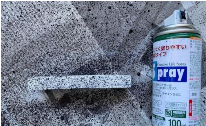
FIGURE 2: Stochastic pattern applied to Koshikake-Aritsugi joint via black spray paint.
